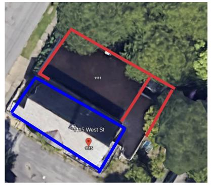
red lines are over view of walls that need to be removed as asbestos to basement floor blue area has already been demoished
